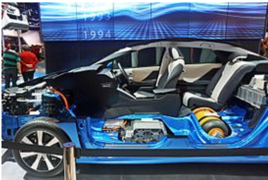
Fig. 1.14 Toyota Mirai fuel cell stack and hydrogen tank (photo from Wikiwand.com)
