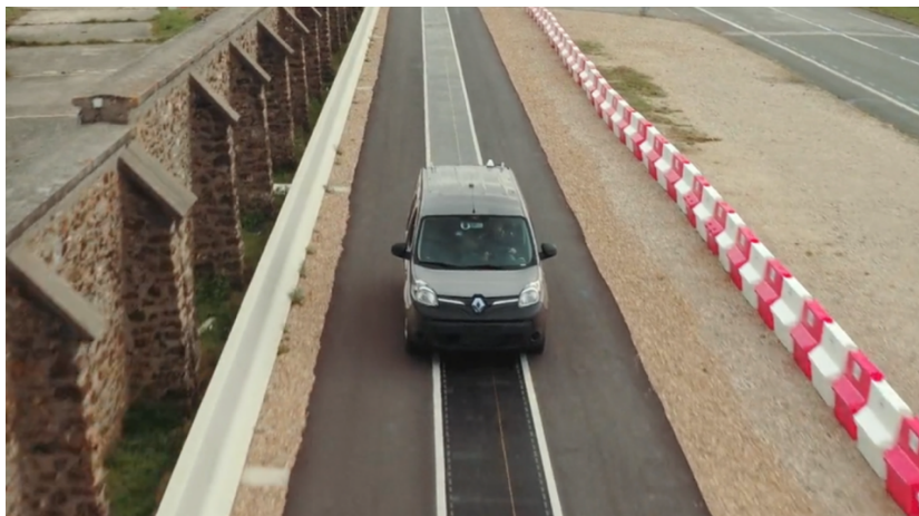
Fig. 1.11 Inductive charging while driving on highway, image Qualcomm , cnet.com/roadshow/, May 2017
