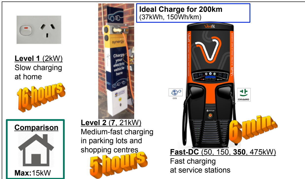
Fig. 1.4 Ideal charging times for home charging, AC slow-charging, DC fast-charging
