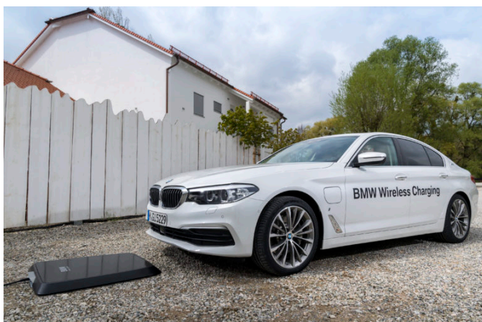
Fig. 1.10 Inductive charging over a plate, [Clean Technica 2018]
