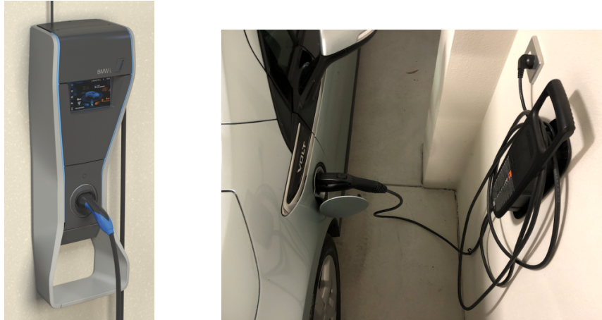
Fig. 1.2 Home charging "wallbox" and "occasional use cable" (photos: BMW, Bräunl)
