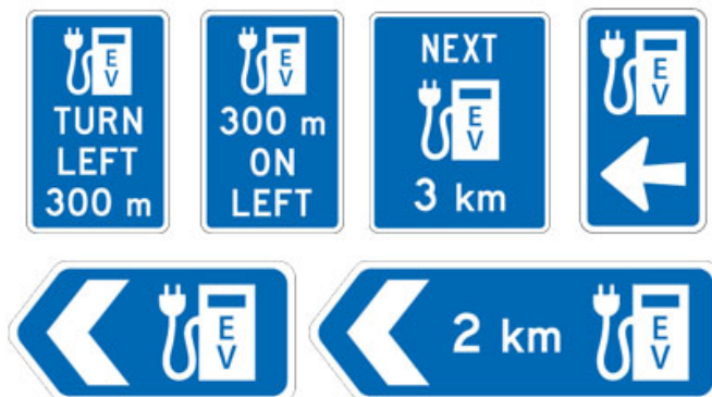
Fig. B.3 Example NZTA way-finding signage (images from [NZTA, 2018])
