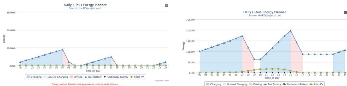
Figure 5-11 Reducing grid power level (left); adding solar PV (right)
