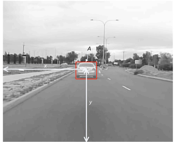
Fig. 2 Figure shows the parameters used in the Kalman filter. They are the coordinates of the vehicle's center point (x,y) and the area of the vehicle's image (A) .
